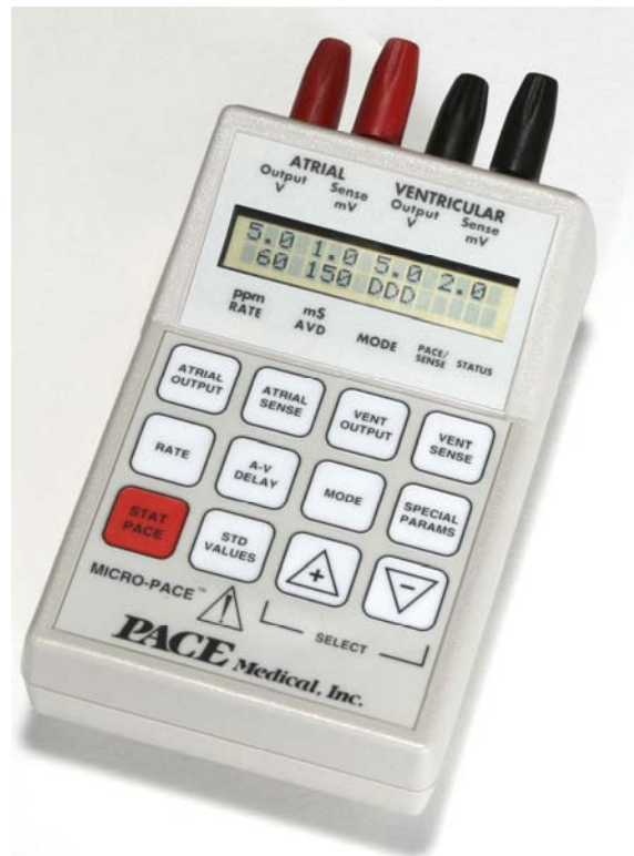
MICRO-PACE Dual-chamber Temporary Cardiac Pacemaker
